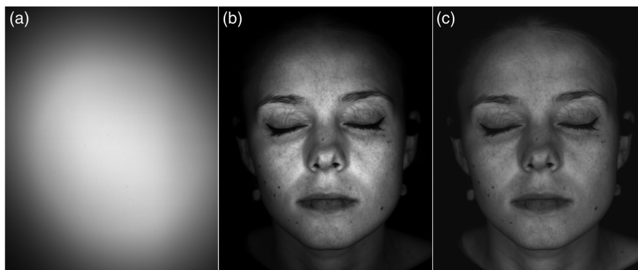
Fig. 2 Acquired and corrected images at 590 nm: (a) nonuniform illumination on the white reference plane, (b) uncalibrated image, and (c) calibrated image.
