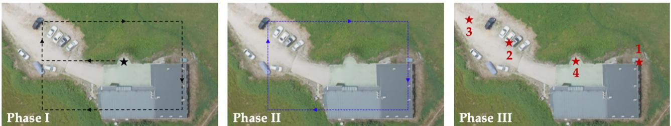
**Fig. 1** The overview of learning the obstacle appearance. Phase I: creating a texton dictionary for the unvisited area based on the captured images during navigation. Phase II: collecting the training data, texton distribution, and surface roughness through the image sequence in the second navigation. Phase III: hovering above the test area (red star) and predicting the surface roughness using the SSL method.
