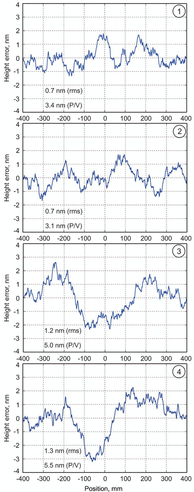
**Fig. 6** Height error traces with a length of 800 mm, obtained as a running sum of the corresponding slope distributions in Fig. 5. The values of the rms and the peak-to-valley height variations are presented on the corresponding plots. Numbers in the circles identify the forecast slope profile in Fig. 5, used for simulation of the corresponding height distribution.
