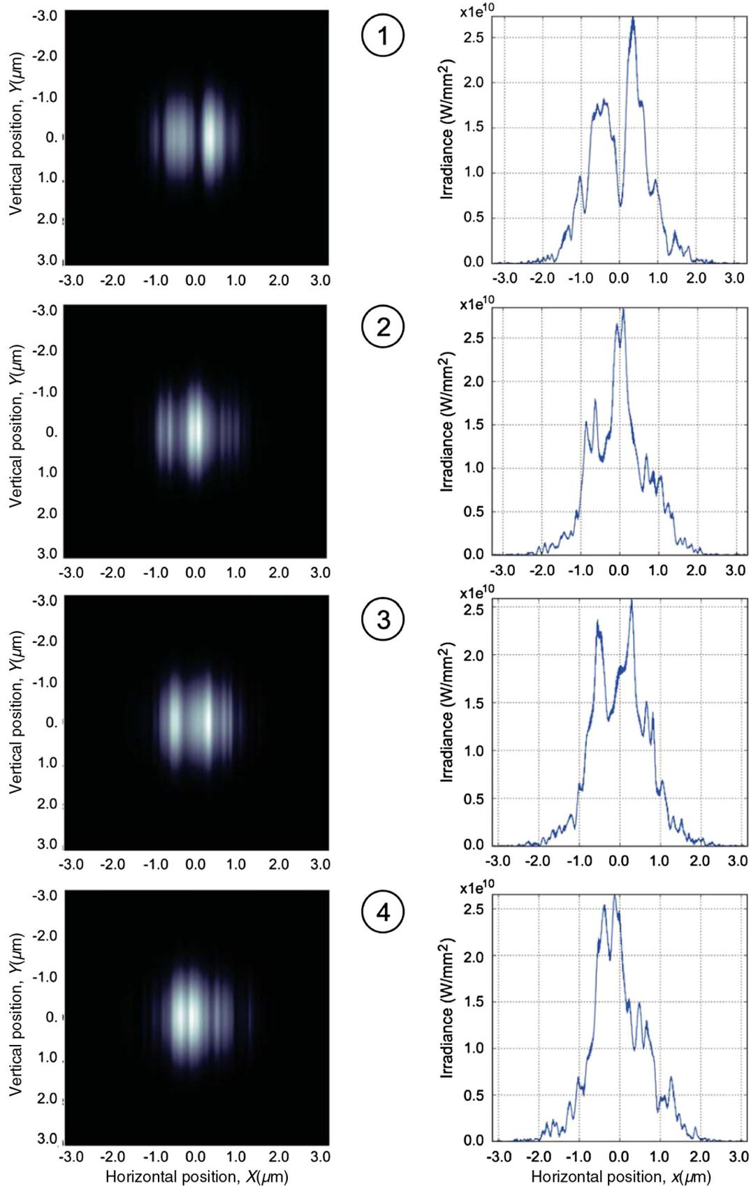
**Fig. 8** Simulated distributions of light irradiance on the entrance aperture of the KB mirror system at 929.6 m from the source: two-dimensional (2-D) distributions (the left-hand set of images) and cross-sections of the 2-D distributions in the horizontal direction at near the vertical position  $Y = 0.0$  mm (the right-hand set of plots). Numbers in the circles identify the forecast slope profile (Fig. 5), used for simulation of the corresponding distribution of light irradiance.
