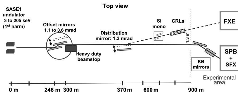
**Fig. 7** The optical scheme of the single particle and bioimaging (SPB) instrument at European XFEL SASE1 beamline: the SPB layout includes two offset mirrors at distances 246 and 258 m, and a 100-nm-scale focusing Kirkpatrick-Baez (KB) system of horizontal and vertical mirrors with focusing distances 3 and 1.9 m, respectively.<sup>61</sup> The KB entrance aperture is at 929.6 m, with incidence angle at 3.5 mrad.
