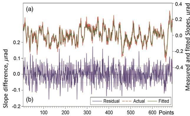
**Fig. 3** (a) Measured slope trace (the red dashed line) after subtracting the best-fitted third polynomial shape in order to remove the trend that is characteristic for short x-ray mirrors, and best-fitted slope trace (the green solid line), corresponding to the ARMA model specified in Table 1. The rms variation of the measured slope trace is 0.0993  $\mu\text{rad}$ . (b) Difference between the measured and fitted traces. The rms variation of the slope difference is 0.0529  $\mu\text{rad}$ .
