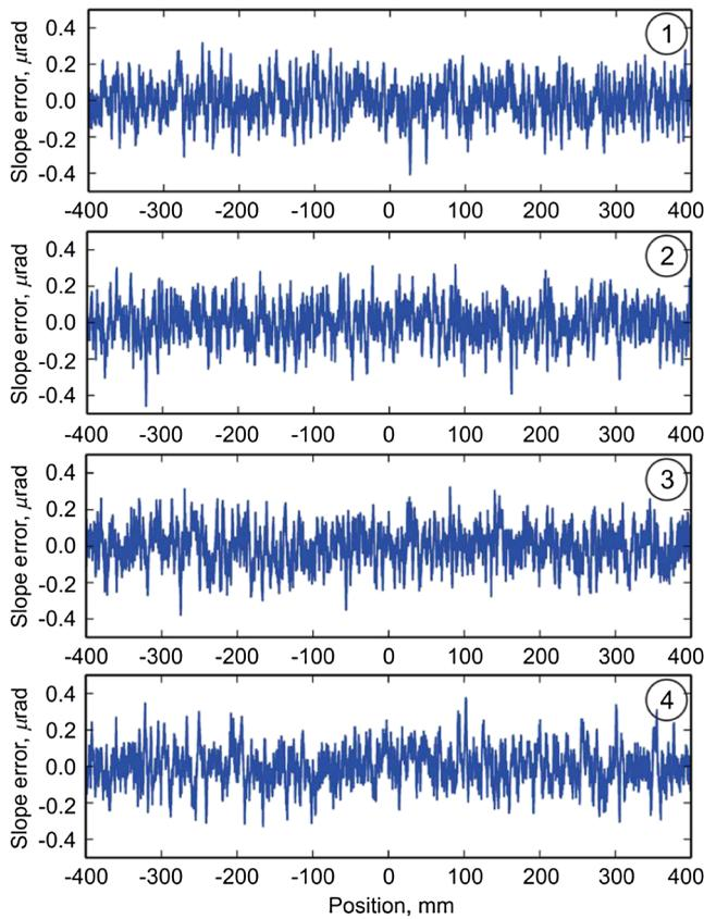
**Fig. 5** Slope error traces with the length of 800 mm, generated with the ARMA model specified in Table 1. The rms slope variation of 0.1  $\mu\text{rad}$  is the same for all traces. Because of the same model parameters used to generate the distributions, the PSD spectra of the traces are also identical.
