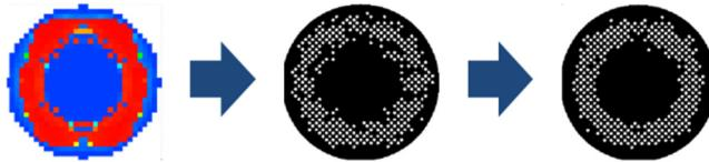
**Fig. 2** The discretization process of a freeform pupil with continuous intensity distribution. The optimal freeform pupil is discretized and optimized into a discrete final pupil, degrading the imaging performance more or less.
