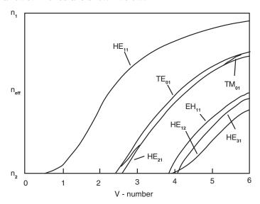
In this figure, the effective-mode index of refraction is  $n_{\rm eff} = (\beta \lambda/2\pi)$ , the V-number is  $V = (2\pi a/\lambda) (n_1^2 - n_2^2)^{1/2}$ , the fiber core radius is a, and  $\beta$  is the mode-propagation constant. Note that this figure shows the allowed mode-propagation constants for a given core radius; for a V-number less than 2.405, only one mode can propagate.
