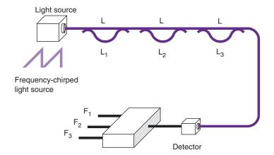
The frequency signal associated with each of the length offsets is then used to separate out each of the successive signals from the Mach–Zehnder (transmission) or Michelson (reflection) interferometers.
