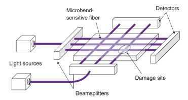
This configuration can also enable safety mats for use with dangerous machinery. Microbend-sensitive optical fibers are woven into the mat, and when an operator is too close to the machinery and steps on the mat, the signal level goes down, and the machinery is switched off. For this simple application, only one light source and detector is needed. The microbend-sensitive optical fiber is wound back and forth through the mat as a single strand.
